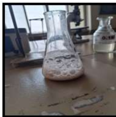
Fig.No.1.6: Foam height test of formulation
